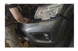
10. Remove the plastic mouldings underneath the headlights.
