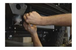
13. There are some hard to find clips that can be popped off with a flat head to remove the rest of the lower air dam.
