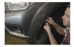
9. Carefully pop the bumper away from the wheel arches and you should be able to pull the whole bumper off now, taking care to disconnect the fog light wiring.
